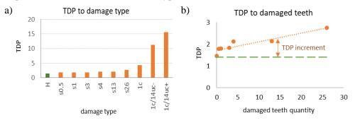
Fig. 4. Diagnostic parameter dependence on damaging (a), damaged teeth quantity (b)
