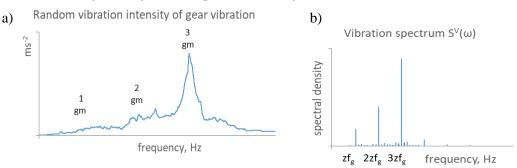
Fig. 2. Vibration of the gear: random component (a), vibration spectrum (b)
